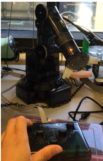
6.115 lab: Control robot arm using keypad
