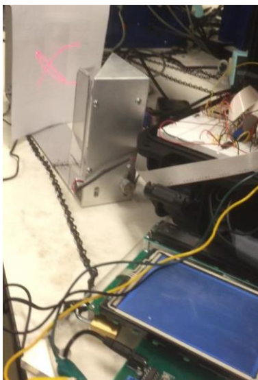
6.115 lab: Using laser pointer to draw picture, controlled by touch screen monitor
